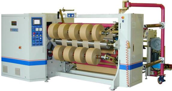
**Application:** 2 shafts center type winding, suitable for slitting/rewinding various label stocks, papers
