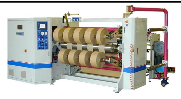
**Application:** 2 shafts center type winding, suitable for slitting/rewinding various adhesive tapes
