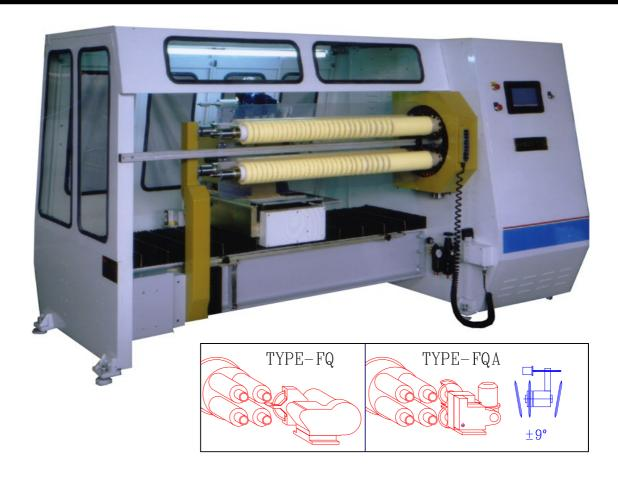
**Application:** Suitable for cutting various adhesive tapes in bulk production.
