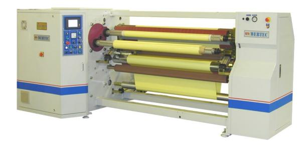
**Application:** 2 shafts auto exchange, suitable for rewinding various self-adhesive tapes.
