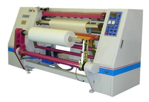
**Application:** Single shaft center-surface type winding, suitable for slitting various adhesive tapes.
