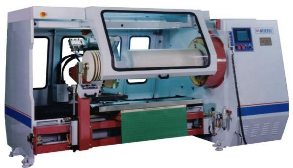
**Application:** Suitable for cutting masking, double side, foam & cloth tapes.
