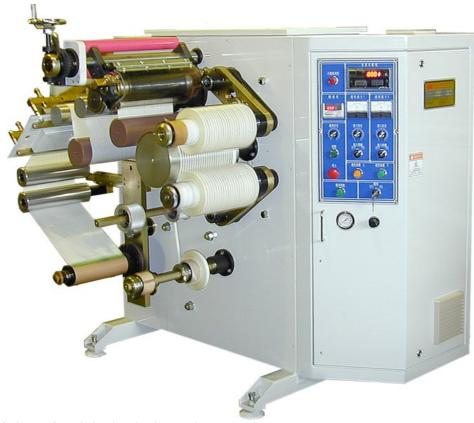
**Application:** Suitable for slitting/rewinding various adhesive tapes.
